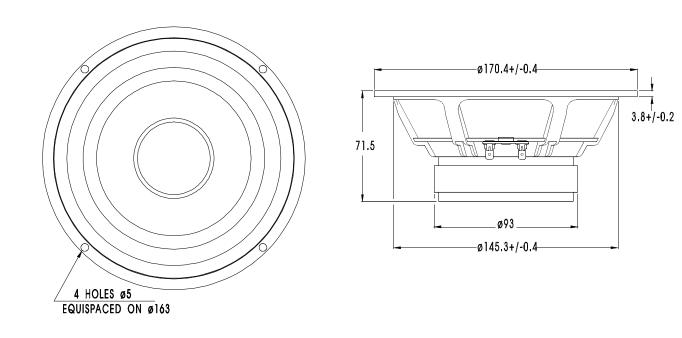
P17RE is a 6,5" High Fidelity woofer with an injection moulded metal chassis. A polypropylene based cone, a soft PVC dust cap and a high loss rubber surround are carefully matched to each other, resulting in an outstandingly smooth frequency response. The unit has a high power handling capacity due to its relatively large voice coil diameter. The magnet system has a T-shaped cross section of the pole piece for low modulation distortion.
