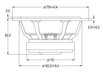
The L18RNX/P is an 18 cm (6,5") cone driver, developed for use as a long throw high fidelity woofer or woofer/midrange unit.
